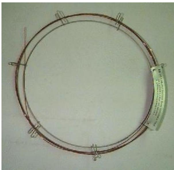
The internal column (capillary)
