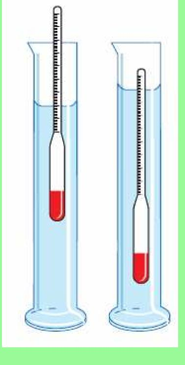
The hydrometer will 'float high' in the grape juice and sink lower as the sugars are converted to alcohol during fermentation. Typically the specific gravity readings for the grape juice will be in the range 1.050-1.120
