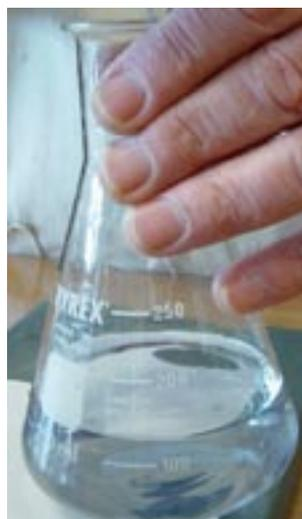
**Figure 5** The endpoint of the titration is reached when just enough thiosulfate is added to react with all the iodine present and the solution becomes colourless.
