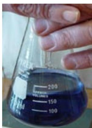
**Figure 3** Upon addition of starch the solution takes on a blue-black colour due to the formation of a starch-iodine complex.
