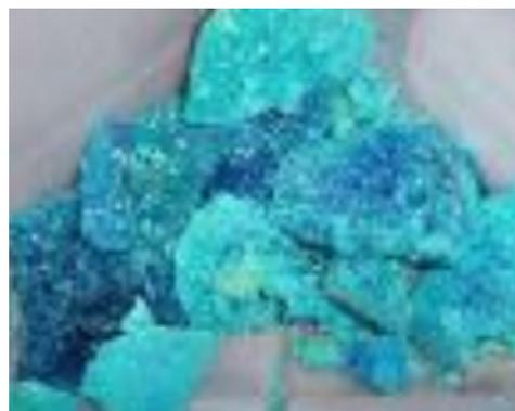
copper sulphate crystals
